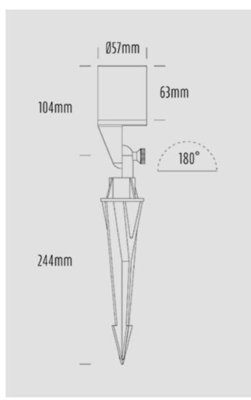
Construction Material Solid Cast Brass
